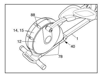
Adjust the position of the Side Shields (14, 15) until the Discs (12) no longer rub against them, and then tighten the Bolt Sets (88) and the M4 x 16mm Screws (78).
